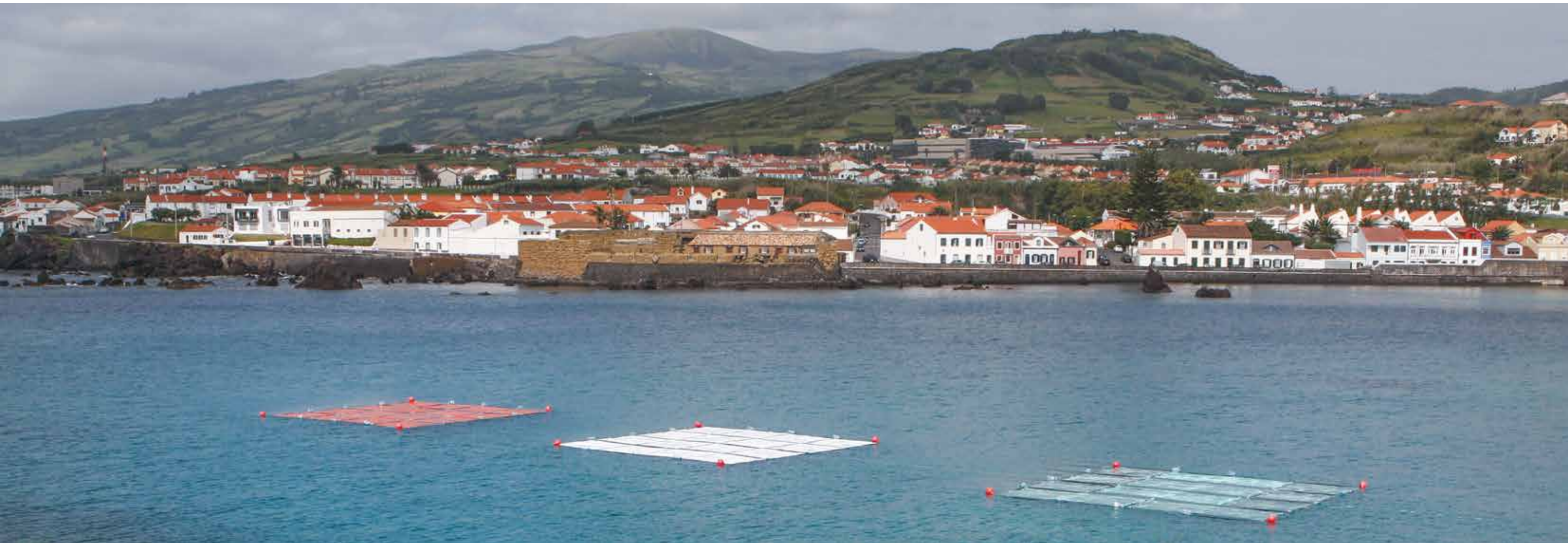
Figure 2 Marine Litter Accumulation Targets for performing development of monitoring technologies using satellite and drone data at Porto Pim, Azores (Photo credits: Hugo Silva)
