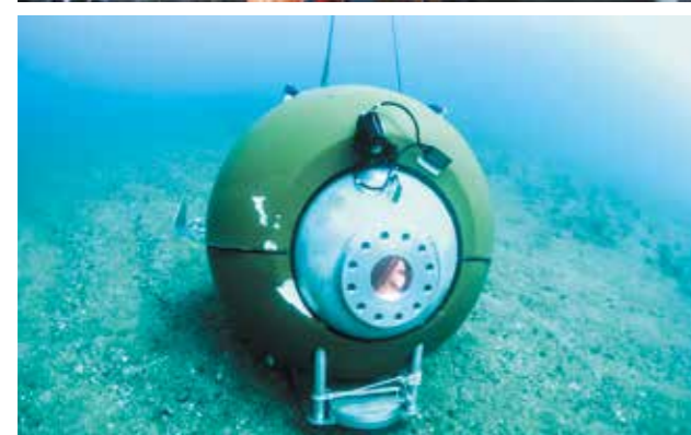
Figure 3 The Hipersea system. The diving chamber attached to the mesopelagic net. The hyperbaric aquarium and the diving chamber at the bottom of the sea. (Photo credits: @Iris)
