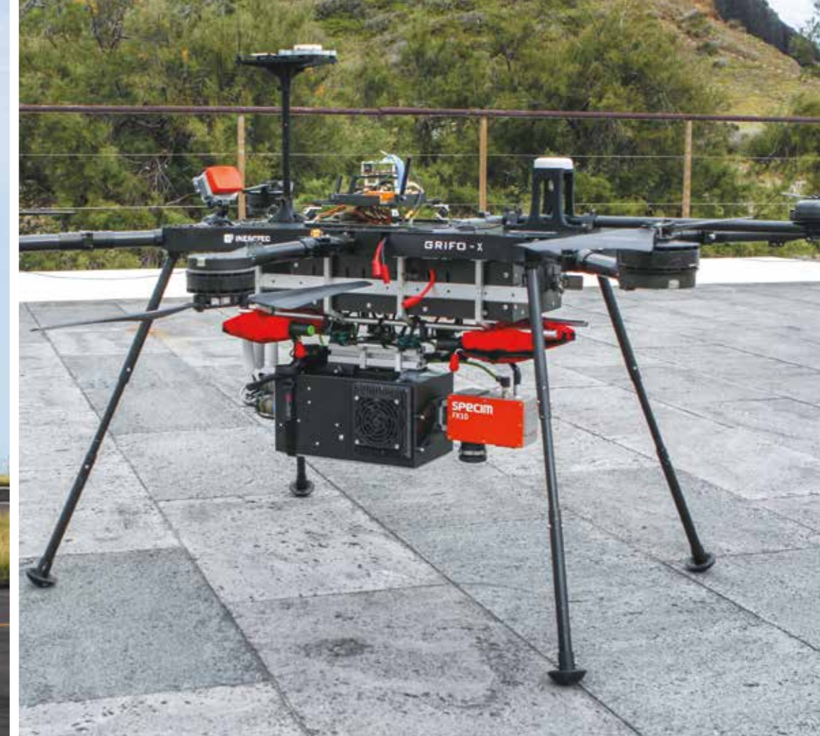
Figure 4 INESC TEC Drone equipped with hyperspectral camera for detecting marine litter during a mission at Porto Pim, Azores (Photo credits: Hugo Silva)
