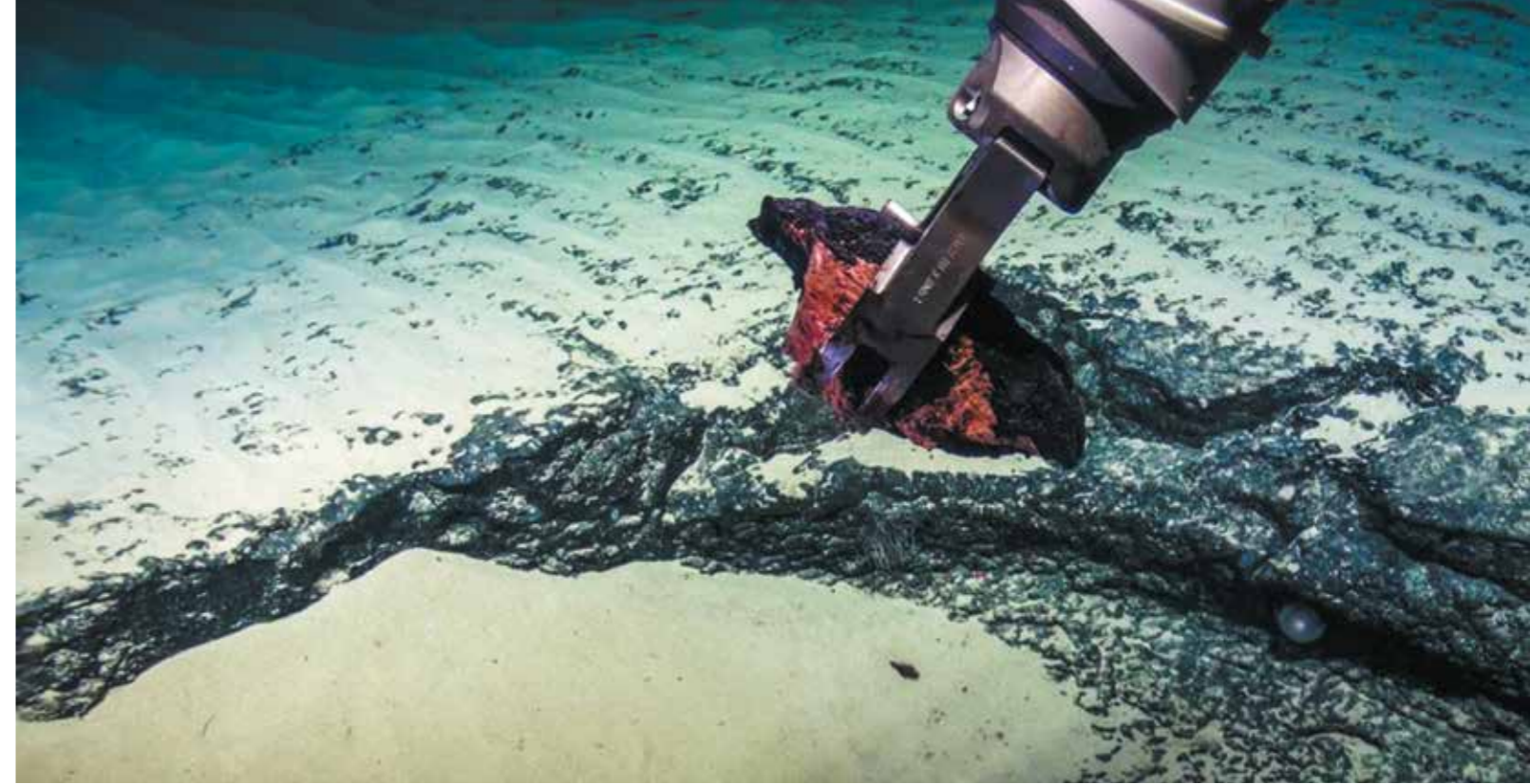
Figure 1 Cobalt-rich crusts being sampled on the summit of Tropic Seamount, NE Atlantic, obtained by remotely operated vehicle. The crust forms a layer of a few tens of cm thick underlain by a substrate of phosphorized carbonate and basalt.
