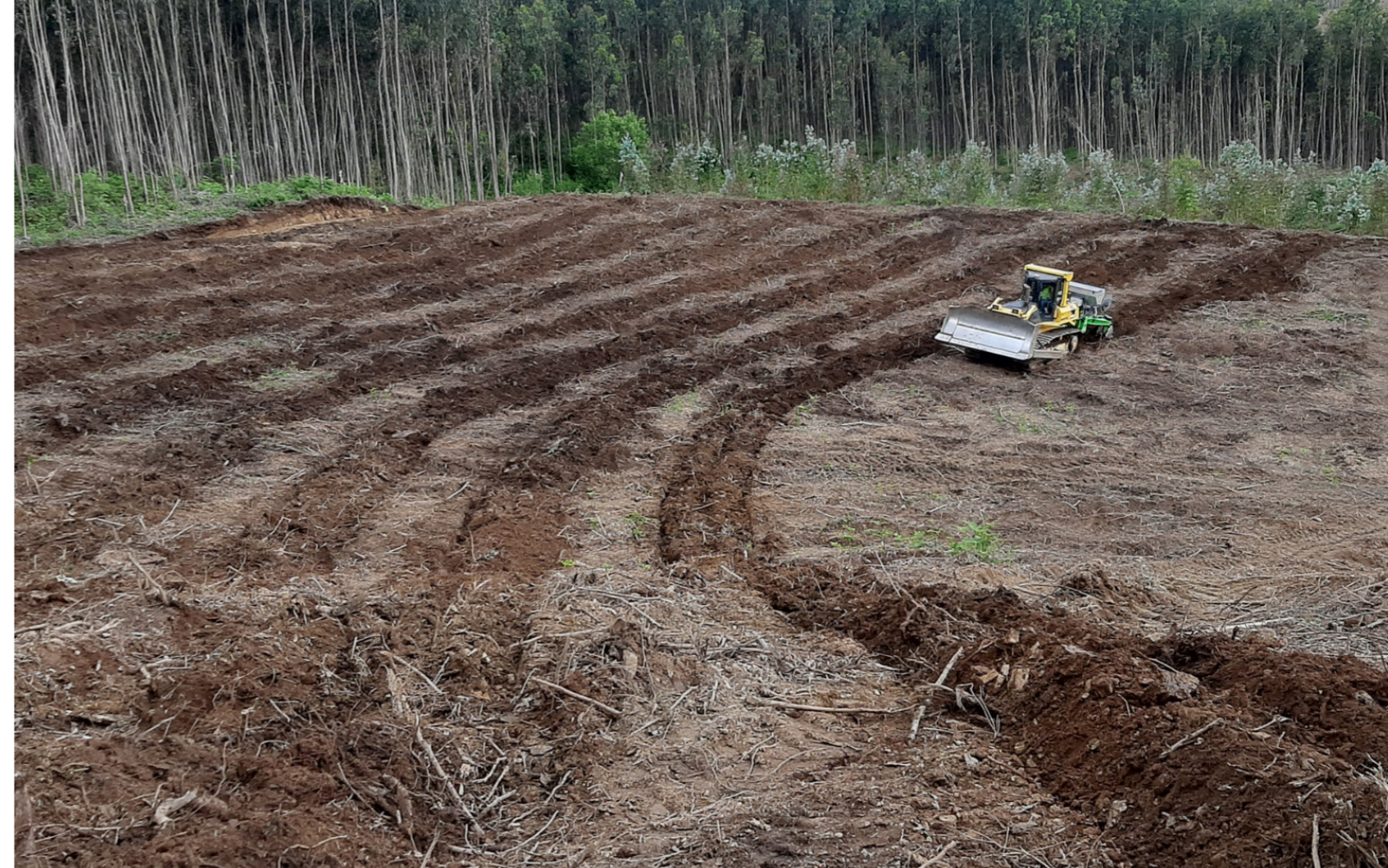
Figure 1 The new ARG forestry machine is based on partial mobilisation for land preparation, promoting plant growth, increasing organic matter conservation, and improving water retention, which contributes to increase soil carbon sequestration. With new Forest 4.0 digital tools, this machine contributes to forest sustainability, as it promotes efficiency and safety of forestry operations with consumption and costs savings and a greater environmental gain. Photo: The Navigator Company and Fravizel (Project rePLANT)
